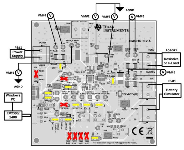
Figure 1. BQ25883 Charge Mode Test Setup
