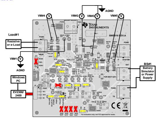
Figure 3. BQ25883 OTG Mode Test Setup
