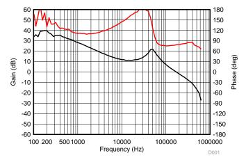
Figure 3. Loop Response ( $V_{IN}$  = 3.6 V,  $V_{OUT}$  = 1.8 V,  $I_{OUT}$  = 750 mA)
