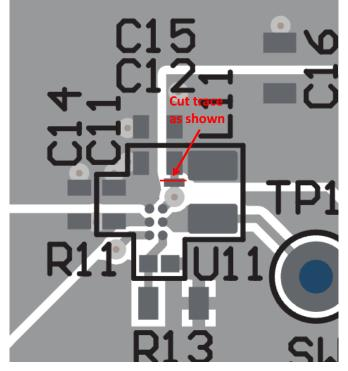
Figure 1. Loop Response Measurement Modification
