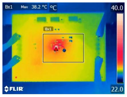
Figure 2. TPS62840 Thermal Performance ( $V_{IN}$  = 3.6 V,  $V_{OUT}$  = 1.8 V,  $I_{OUT}$  = 750 mA)
