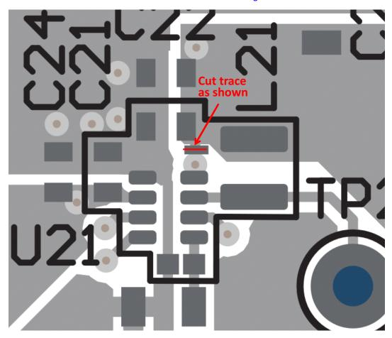
Figure 1. Loop Response Measurement Modification
