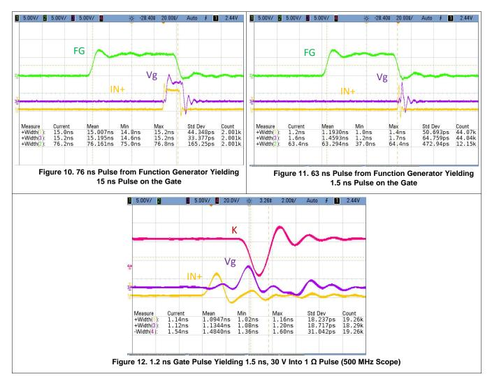
Figure 10 through Figure 11 show how the input stage performs and how the buffer cleans up and shortens the input pulse. This allows the use of a function generator with lower specifications.
