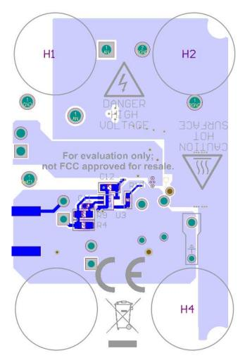
Figure 14. LMG1025-Q1EVM Bottom Layer and Components
