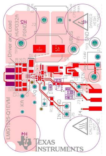
Figure 13. LMG1025-Q1EVM Top Layer and Components
