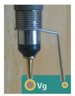
Figure 7. Recommended Use for Ground Spring Clip Test Points
