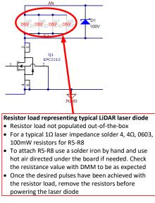
Figure 3. Schematic View of Unpopulated Load Resistors R5–R8
