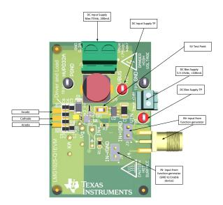
Figure 6. Recommended Connection Points and Feature Description
