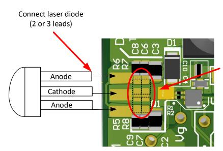
Out-of-the-box, the resistor load is not populated. With no laser diode connected, for out-of-the-box power loop functionality, solder the resistive laser load consisting of 4 parallel 0603, 100mW resistors (R5-R8). Remove resistor load before using laser diode
