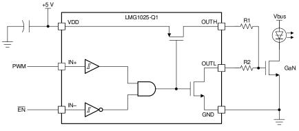
Figure 2. LiDAR Power Stage with LMG1025-Q1
