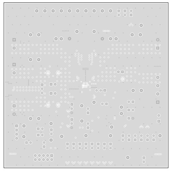
Figure 4-4. BMS027A Signal Layer 1
