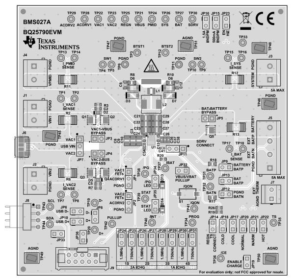
Figure 4-3. BMS027A Top Layer and Overlay
