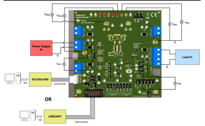
Figure 2-1. Equipment Test Setup for BMS027A
