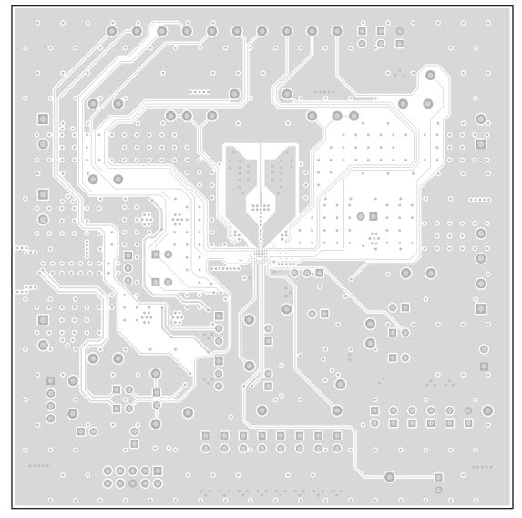
Figure 4-5. BMS027A Signal Layer 2
