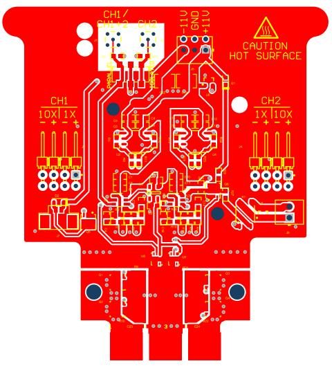
Figure 4. Top Assembly Layer
