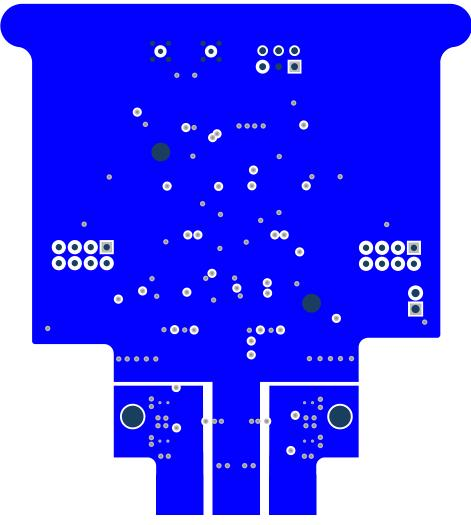
Figure 8. Bottom Layer Routing
