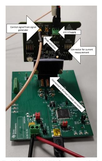
Figure 3. The PMICLOADBOARDEVM Connected to LP875701Q1EVM
