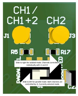
Figure 2. Switch S1 Control Selection
