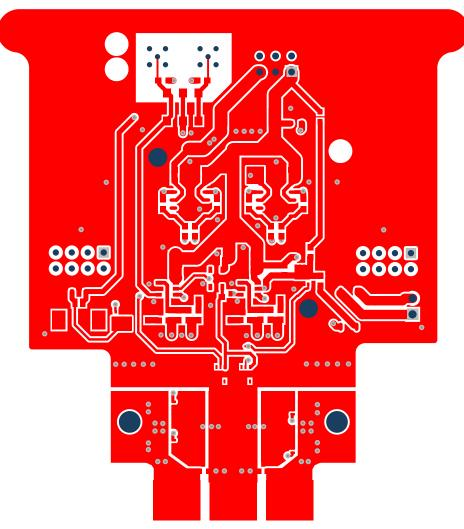
Figure 5. Top Layer Routing
