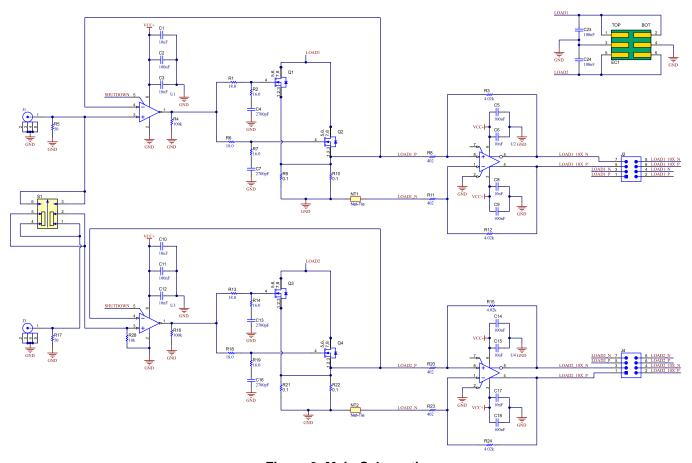
Figure 9. Main Schematic
