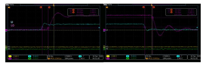
Figure 4. LI and LO Propagation Delay Waveforms (Green and Magenta are PWM Inputs, Yellow and Blue are Driver Outputs)
