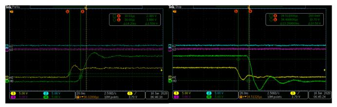
Figure 3. HI and HO Propagation Delay Waveforms (Green and Magenta are PWM Inputs, Yellow and Blue are Driver Outputs)
