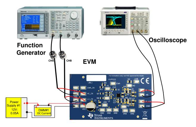
Figure 1. Bench Setup Diagram and Configuration
