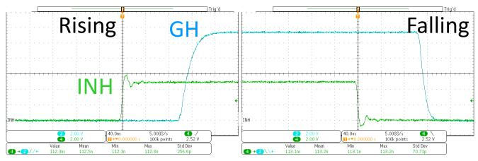
Figure 7-1. INH and GH Propagation Delay Waveforms (green is INH, blue is GH)
