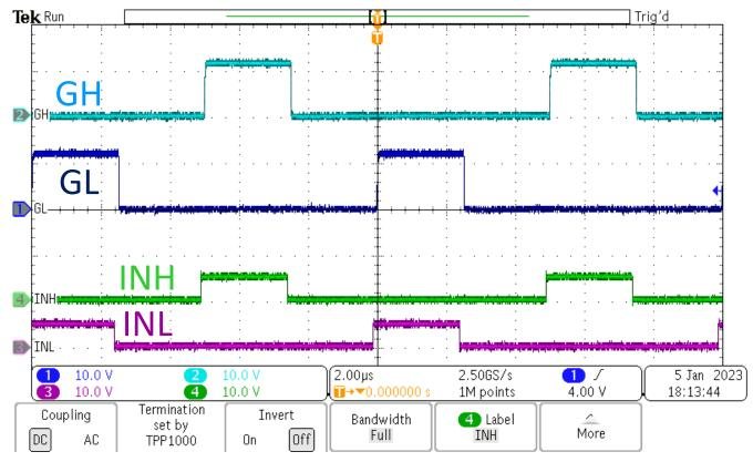
Figure 5-1. Example Input and Output Waveforms (green and magenta are PWM inputs, blue and dark blue are driver outputs)
