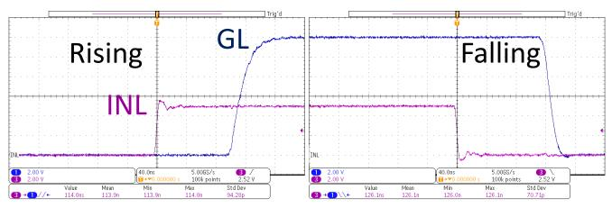
Figure 7-2. INL and GL Propagation Delay Waveforms (green is GL, dark blue is GL)
