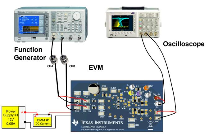
Figure 4-1. Bench Setup Diagram and Configuration
