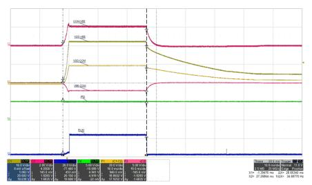
Figure 5-22. Output UVLO, PVDD=0 mW, PVEE=313 mW, (top: COM-VEE, 2 V/div, mid1: VDD-VEE, 10 V/div, mid2: VDD-COM, 20 V/div, mid3: VEE-COM, 5 V/div, bot: RLIM, 20 V/div), time = 10 ms/div
