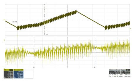
Figure 5-17. AC Ripple: VIN=12 V, IVDD=68 mA, FBURST=1 MHz (VDD-VEE, 50 mV/div, Zoom: VDD-VEE, 10 mV/div), time = 5 µs/div, time\_zoom=200 ns/div
