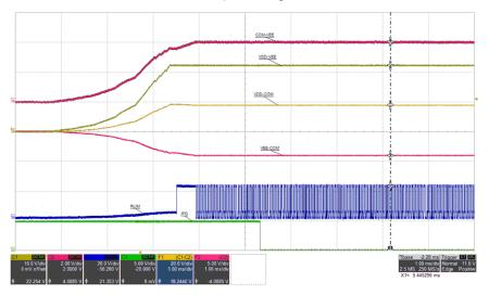
Figure 5-24. Normal Start, VIN=12 V, PVDD=324 mW, PVEE=106 mW, (top: COM-VEE, 2 V/div, mid1: VDD-VEE, 10 V/div, mid2: VDD-COM, 20 V/div, mid3: VEE-COM, 5 V/div, mid4: RLIM, 20 V/div, bot: /PG, 5 V/div), time = 1 ms/div
