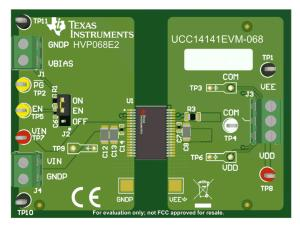
Figure 6-1. UCC14141EVM-068, Fully Assembled 3D Top View
