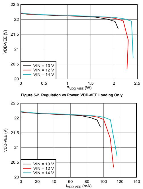
Figure 5-3. Regulation vs Current, VDD-VEE Loading Only
