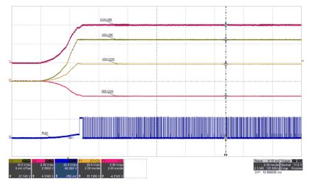
Figure 5-20. RLIM: VIN=12 V, I<sub>VDD-VEE</sub>=68 mA, (top: COM-VEE, 2 V/div, mid-1: VDD-VEE, 10 V/div, mid-2: VDD-COM, 20 V/div, mid-3: VEE-COM, 5 V/div, bot: RLIM, 20 V/div), time = 2 ms/div
