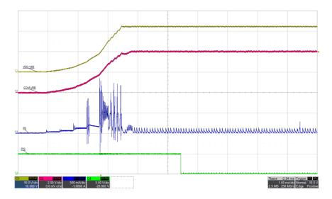
Figure 5-11. Inrush Current: VIN=12 V, I<sub>VDD-VEE</sub>=0 mA, (top: VDD-VEE, 10 V/div, mid-1: COM-VEE, 2 V/div, mid-2: IIN, 0.5 A/div, bot: /PG, 5 V/div), time = 1 ms/div
