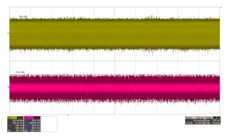
Figure 5-13. VDD<sub>AC</sub>=240 mV, VEE<sub>AC</sub>=100 mV,  $I_{VDD}$ =68 mA,  $I_{VEE}$ =30 mA (top: VDD-VEE, 100 mV/div, bot: COM-VEE, 50 mV/div), time = 100 ms/div
