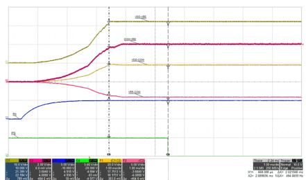
Figure 5-8. Start-up 4: VIN=12 V, I<sub>VDD-VEE</sub>=68 mA, (top: VDD-VEE, 10 V/div, mid-1: COM-VEE, 2 V/div, mid-2: VDD-COM, 20 V/div, mid-3: VEE-COM, 5 V/div, mid-4: EN, 5 V/div, bot: /PG, 5 V/div), time = 1 ms/div
