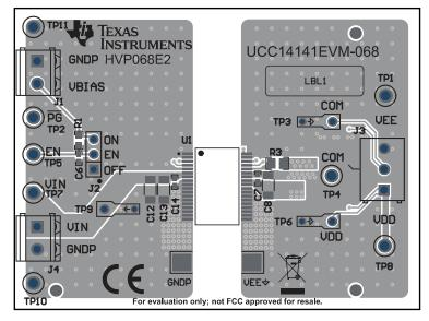
Figure 6-4. UCC14141EVM-068, PCB Top Layer, Assembly
