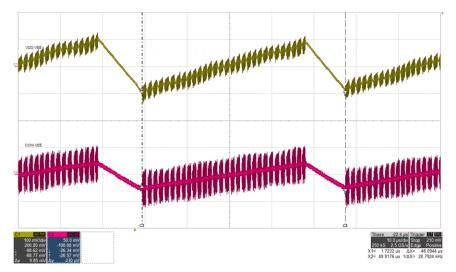
Figure 5-15. AC Ripple: VIN=12 V, IVDD=68 mA, IVEE=30 mA, FMOD=20.8 kHz (top: VDD-VEE, 100 mV/div, bot: COM-VEE, 50 mV/div), time = 10 µs/div
