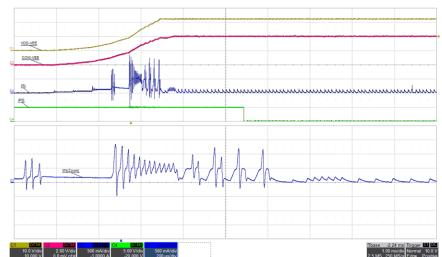
Figure 5-12. Inrush Current: VIN=12 V, I<sub>VDD-VEE</sub>=68 mA, (top: VDD-VEE, 10 V/div, mid-1: COM-VEE, 2 V/div, mid-2: IIN, 0.5 A/div, bot: /PG, 5 V/div), time = 1 ms/div, time\_zoom=200 µs/div
