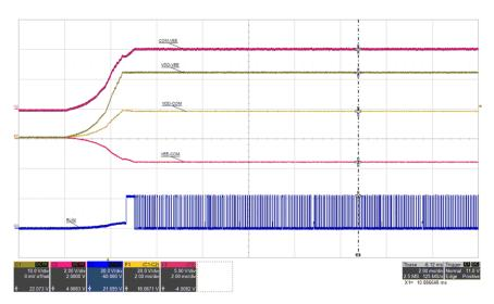
Figure 5-19. RLIM: VIN=12 V, I<sub>VDD-VEE</sub>=0 mA, (top: COM-VEE, 2 V/div, mid-1: VDD-VEE, 10 V/div, mid-2: VDD-COM, 20 V/div, mid-3: VEE-COM, 5 V/div, bot: RLIM, 20 V/div), time = 2 ms/div
