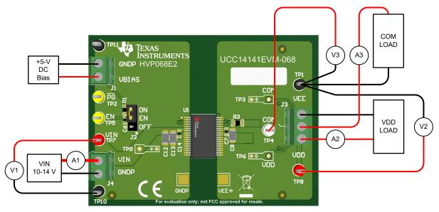
Figure 4-1. Typical Efficiency Measurement Setup
