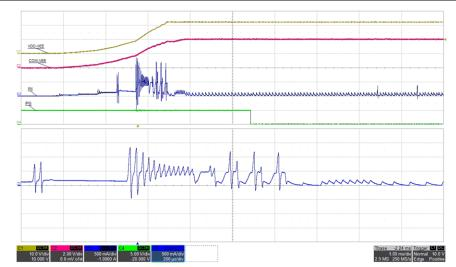
Figure 5-10. Inrush Current: VIN=12 V, I<sub>VDD-VEE</sub>=68 mA, (top: VDD-VEE, 10 V/div, mid-1: COM-VEE, 2 V/div, mid-2: IIN, 0.5 A/div, bot: /PG, 5 V/div), time = 1 ms/div, time\_zoom=200 µs/div
