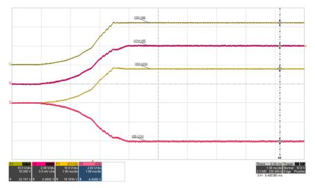
Figure 5-5. Start-up 1: VIN=12 V, I<sub>VDD-VEE</sub>=0 mA, (top: VDD-VEE, 10 V/div, mid-1: COM-VEE, 2 V/div, mid-2: VDD-COM, 10 V/div, bot: VEE-COM, 2 V/div), time = 1 ms/div
