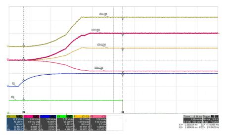
Figure 5-7. Start-up 3: VIN=12 V, I<sub>VDD-VEE</sub>=68 mA, (top: VDD-VEE, 10 V/div, mid-1: COM-VEE, 2 V/div, mid-2: VDD-COM, 20 V/div, mid-3: VEE-COM, 5 V/div, mid-4: EN, 5 V/div, bot: /PG, 5 V/div), time = 1 ms/div
