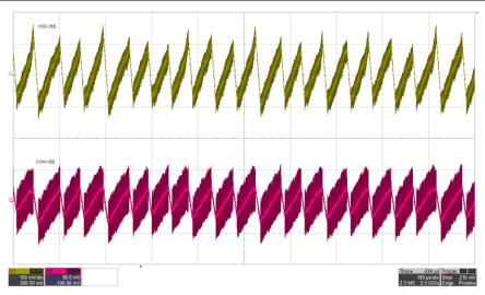
Figure 5-14. AC Ripple: VIN=12 V, IVDD=68 mA, IVEE=30 mA (top: VDD-VEE, 100 mV/div, bot: COM-VEE, 50 mV/div), time = 100 µs/div
