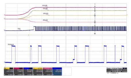
Figure 5-21. RLIM: VIN=12 V, I<sub>VDD-VEE</sub>=68 mA, (top: COM-VEE, 2 V/div, mid-1: VDD-VEE, 10 V/div, mid-2: VDD-COM, 20 V/div, mid-3: VEE-COM, 5 V/div, bot: RLIM, 20 V/div, Zoom: RLIM, 5 V/div), time = 10 ms/div, time\_zoom = 50 µs/div
