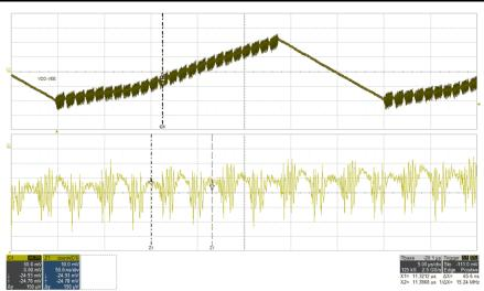
Figure 5-16. AC Ripple: VIN=12 V, IVDD=68 mA, FSW(PRI)=15.24 kHz (VDD-VEE, 50 mV/div, Zoom: VDD-VEE, 10 mV/div), time = 5 µs/div, time\_zoom=50 ns/div
