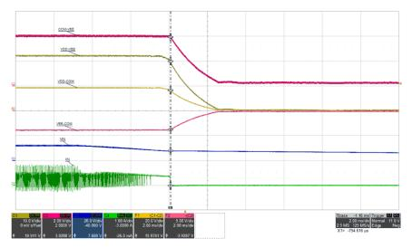
Figure 5-25. Shutdown by VIN Removal: VIN<sub>OFF</sub>=7.6 V, I<sub>VDD-VEE</sub>=68 mA (top: COM-VEE, 2 V/div, mid-1: VDD-VEE, 10 V/div, mid-2: VDD-COM, 20 V/div, mid-3: VEE-COM, 5 V/div, mid-4: VIN, 20 V/div, bot: IIN, 1 A/div), time = 2 ms/div
