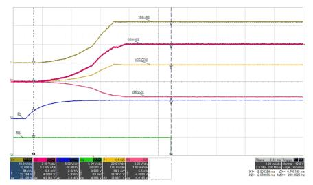
Figure 5-18. ENA to /PG Delay, 4.7 ms, I<sub>VDD-VEE</sub>=68 mA, (top: VDD-VEE, 10 V/div, mid1: COM-VEE, 2 V/div, mid2: VDD-COM, 20 V/div, mid3: VEE-COM, 5 V/div, mid4: EN, 5 V/div, bot: /PG, 5 V/div), time = 1 ms/div
