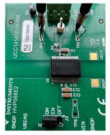
Figure 4-2. UCC14141EVM-068, PCB Scope Probe Test Points
