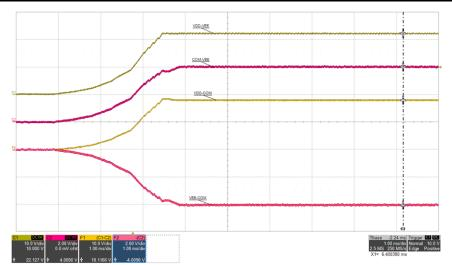
Figure 5-6. Start-up 2: VIN=12 V, I<sub>VDD-VEE</sub>=68 mA, (top: VDD-VEE, 10 V/div, mid-1: COM-VEE, 2 V/div, mid-2: VDD-COM, 10 V/div, bot: VEE-COM, 2 V/div), time = 1 ms/div
