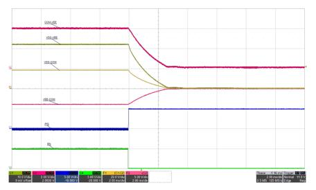
Figure 5-26. Shutdown by EN Low: VIN=12 V, I<sub>VDD-VEE</sub>=68 mA, (top: COM-VEE, 2 V/div, mid-1: VDD-VEE, 10 V/div, mid-2: VDD-COM, 20 V/div, mid-3: VEE-COM, 5 V/div, mid-4: /PG, 5 V/div, bot: ENA, 5 V/div), time = 2 ms/div
