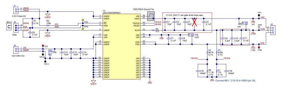
Figure 3-1. UCC14341EVM-069 Schematic Diagram
