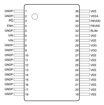
Figure 1-1. DWN Package, 36-Pin SSOP (Top View)
