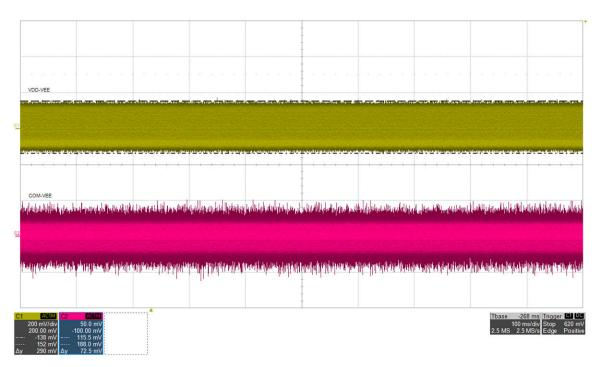
Figure 5-12. AC Ripple 1:  $VDD_{AC}$ =290 mV,  $VEE_{AC}$ =90 mV,  $I_{VDD}$ =68 mA,  $I_{VEE}$ =0 mA (top: VDD-VEE, 200 mV/div), bot:  $VEE_{AC}$ =100 mS/div
