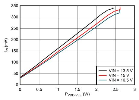
Figure 5-4. Input Current vs Power, VDD-VEE Loading Only
