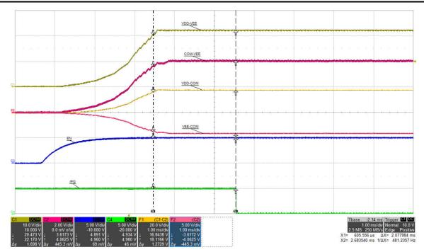
Figure 5-8. Start-up 4: VIN=15 V, I<sub>VDD-VEE</sub>=68 mA, (top: VDD-VEE, 10 V/div, mid-1: COM-VEE, 2 V/div, mid-2: VDD-COM, 20 V/div, mid-3: VEE-COM, 5 V/div, mid-4: EN, 5 V/div, bot: /PG, 5 V/div), time = 1 ms/div, Reg to /PG delay = 2.07 ms
