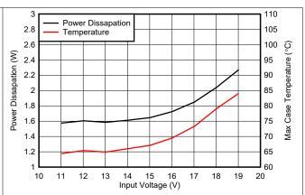
Figure 5-28. Power Dissipation and Case Temperature vs Input Voltage, T<sub>A</sub>=23°C, 1.51 W
