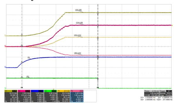
Figure 5-17. ENA to /PG Delay, 4.6 ms, VIN=15 V, I<sub>VDD-VEE</sub>=68 mA, (top: VDD-VEE, 10 V/div, mid-1: COM-VEE, 2 V/div, mid-2: VDD-COM, 20 V/div, mid-3: VEE-COM, 5 V/div, mid-4: EN, 5 V/div, bot: /PG, 5 V/div), time = 1 ms/div
