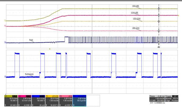
Figure 5-20. RLIM 3: VIN=15 V, I<sub>VDD-VEE</sub>=68 mA, (top: VDD-VEE, 10 V/div, mid-1: COM-VEE, 2 V/div, mid-2: VDD-COM, 20 V/div, mid-3: VEE-COM, 5 V/div, bot: RLIM, 20 V/div, Zoom: RLIM, 5 V/div), time = 1 ms/div, time\_zoom = 50 μs/div
