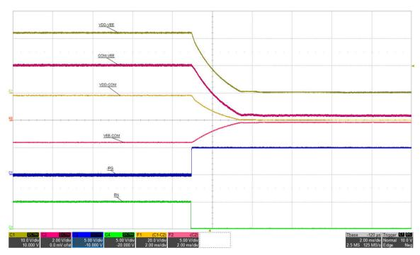
Figure 5-25. Shutdown by EN Low: VIN=15 V, I<sub>VDD-VEE</sub>=68 mA (top: VDD-VEE, 10 V/div, mid-1: COM-VEE, 2 V/div, mid-2: VDD-COM, 20 V/div, mid-3: VEE-COM, 5 V/div, mid-4: /PG, 5 V/div, bot: EN, 5 V/div), time=2 ms/div
