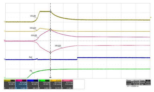
Figure 5-22. COM-VEE OVP: VIN=15 V, PVDD=188 mW, PVEE=0 mW, (top: VDD-VEE, 20 V/div, mid-1: VDD-COM, 50 V/div, mid-2: COM-VEE, 10 V/div, mid-3: VEE-COM, 10 V/div, mid-4: RLIM, 20 V/div, bot: /PG, 5 V/div), time = 5 ms/div
