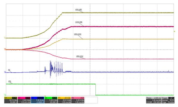
Figure 5-9. Inrush Current 1: VIN=15 V, I<sub>VDD-VEE</sub>=68 mA, (top: VDD-VEE, 10 V/div, mid-1: COM-VEE, 2 V/div, mid-2: VDD-COM, 20 V/div, mid-3: VEE-COM, 5 V/div, mid-4: IIN, 1 A/div, bot: /PG, 5 V/div), time = 1 ms/div
