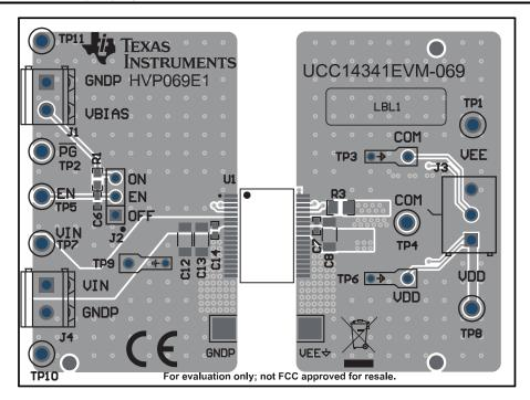
Figure 6-4. UCC14341EVM-069, PCB Top Layer, Assembly
