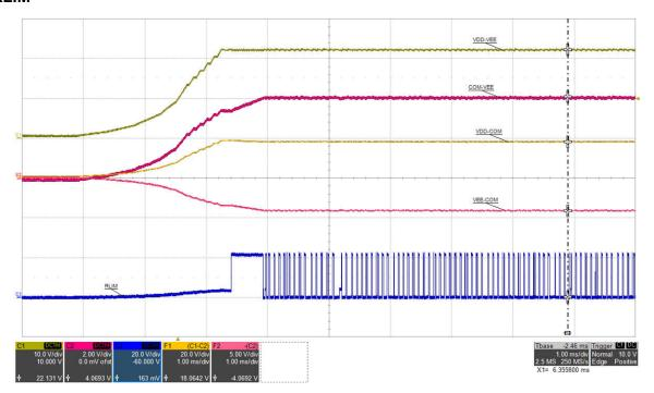
Figure 5-18. RLIM 1: VIN=15 V, I<sub>VDD-VEE</sub>=0 mA, (top: VDD-VEE, 10 V/div, mid-1: COM-VEE, 2 V/div, mid-2: VDD-COM, 20 V/div, mid-3: VEE-COM, 5 V/div, bot: RLIM, 20 V/div), time = 1 ms/div
