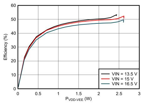
Figure 5-1. Measured Efficiency, VDD-VEE Loading Only
