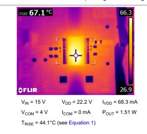
Figure 5-27. VIN=15 V, I<sub>VDD-VEE</sub>=68.3 mA, 1.51 W
