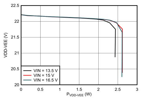
Figure 5-2. Regulation vs Power, VDD-VEE Loading Only
