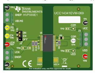
Figure 6-1. UCC14341EVM-069, Fully Assembled 3D Top View
