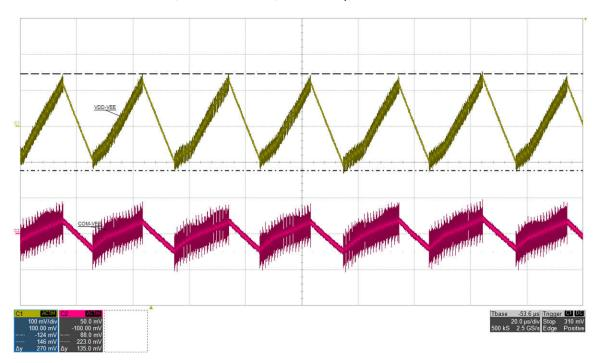
Figure 5-13. AC Ripple 2: VIN=15 V, IVDD=68 mA, IVEE=0 mA, (top: VDD-VEE, 100 mV/div, bot: COM-VEE, 50 mV/div), time = 20  $\mu$ s/div
