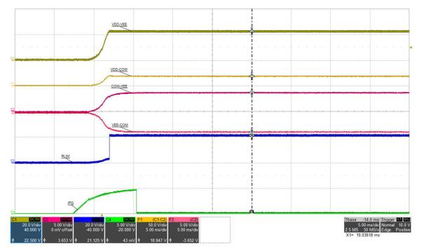
Figure 5-23. Normal Start (close to COM-VEE UVLO): VIN=15 V, PVDD=573 mW, PVEE=404 mW, (top: VDD-VEE, 20 V/div, mid-1: VDD-COM, 50 V/div, mid-2: COM-VEE, 5 V/div, mid-3: VEE-COM, 5 V/div, mid-4: RLIM, 20 V/div, bot: /PG, 5 V/div), time = 5 ms/div
