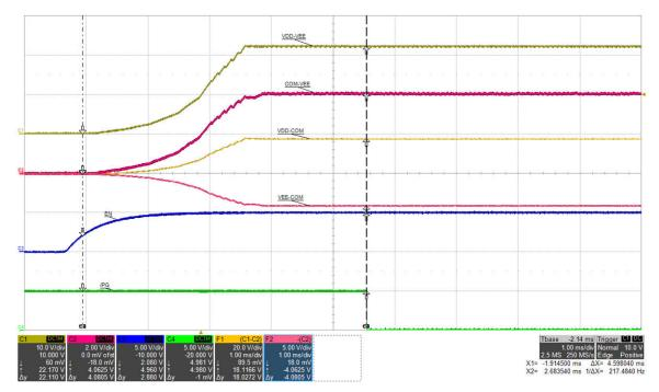
Figure 5-7. Start-up 3: VIN=15 V, I<sub>VDD-VEE</sub>=68 mA, (top: VDD-VEE, 10 V/div, mid-1: COM-VEE, 2 V/div, mid-2: VDD-COM, 20 V/div, mid-3: VEE-COM, 5 V/div, mid-4: EN, 5 V/div, bot: /PG, 5 V/div), time = 1 ms/div, EN to /PG delay = 4.6 ms
