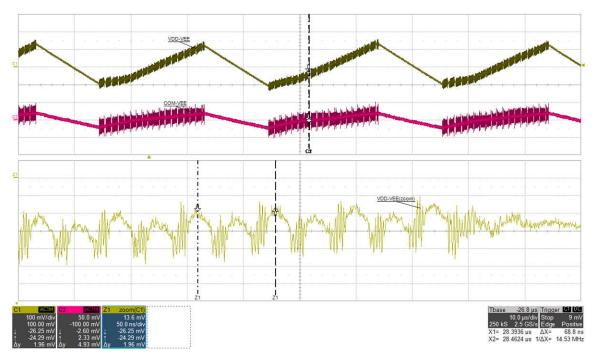
Figure 5-15. AC Ripple 4: VIN=15 V, IVDD=68 mA, FSW(PRI)=14.53 MHz, (top: VDD-VEE, 100 mV/div, bot: COM-VEE, 50 mV/div, Zoom: VDD-VEE, 13.6 mV/div), time =10 µs/div, time\_zoom=50 ns/div
