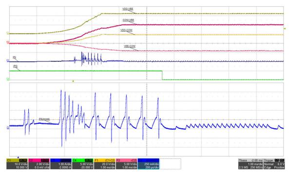
Figure 5-11. Inrush Current 3: VIN=15 V, I<sub>VDD-VEE</sub>=0 mA, (top: VDD-VEE, 10 V/div, mid-1: COM-VEE, 2 V/div, mid-2: VDD-COM, 20 V/div, mid-3: VEE-COM, 5 V/div, mid-4: IIN, 1 A/div, bot: /PG, 5 V/div, zoom: 250 mA/div), time =1 ms/div, time\_zoom=200 μs/div
