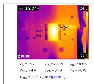
Figure 5-29. VIN=15 V, I<sub>VDD-VEE</sub>=0 mA, POUT=0 W
