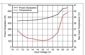
Figure 5-30. Power Dissipation and Case Temperature vs Input Voltage, TA=23°C, 0 W
