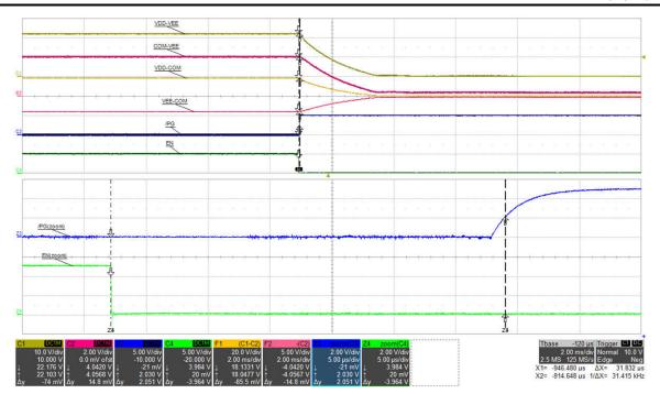
Figure 5-26. Shutdown by EN Low (zoom): VIN=15 V, I<sub>VDD-VEE</sub>=68 mA (top: VDD-VEE, 10 V/div, mid-1: COM-VEE, 2 V/div, mid-2: VDD-COM, 20 V/div, mid-3: VEE-COM, 5 V/div, mid-4: /PG, 5 V/div, bot: EN, 5 V/div, top\_zoom: /PG, 2 V/div, bot\_zoom: EN, 2 V/div), time=2 ms/div, time\_zoom=5 μs/div
