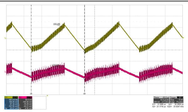
Figure 5-14. AC Ripple 3: VIN=15 V, IVDD=68 mA, IVEE=0 mA, FMOD=33 kHz, (top: VDD-VEE, 100 mV/div, bot: COM-VEE, 50 mV/div), time =10 µs/div
