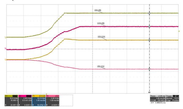
Figure 5-5. Start-up 1: VIN=15 V, I<sub>VDD-VEE</sub>=0 mA, (top: VDD-VEE, 10 V/div, mid-1: COM-VEE, 2 V/div, mid-2: VDD-COM, 10 V/div, bot: VEE-COM, 5 V/div), time = 1 ms/div
