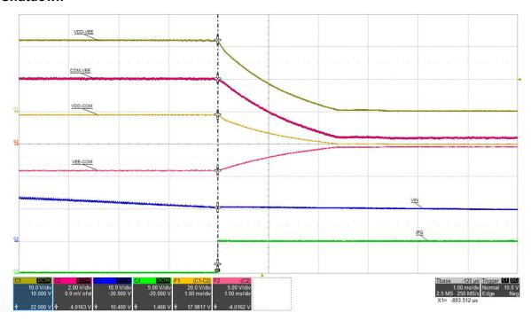
Figure 5-24. Shutdown by VIN Removal: VIN<sub>OFF</sub>=10.4 V, I<sub>VDD-VEE</sub>=68 mA (top: VDD-VEE, 10 V/div, mid-1: COM-VEE, 2 V/div, mid-2: VDD-COM, 20 V/div, mid-3: VEE-COM, 5 V/div, mid-4: VIN, 10 V/div, bot: /PG, 5 V/div), time=1 ms/div
