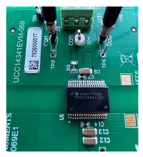
Figure 4-2. UCC14341EVM-069, PCB Scope Probe Test Points
