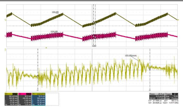
Figure 5-16. AC Ripple 5: VIN=15 V, IVDD=68 mA, FBURST=1 MHz, (top: VDD-VEE, 100 mV/div, bot: COM-VEE, 50 mV/div, Zoom: VDD-VEE, 10 mV/div), time =10 µs/div, time\_zoom=150 ns/div
