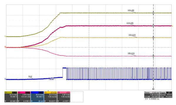
Figure 5-19. RLIM 2: VIN=15 V, I<sub>VDD-VEE</sub>=68 mA, (top: VDD-VEE, 10 V/div, mid-1: COM-VEE, 2 V/div, mid-2: VDD-COM, 20 V/div, mid-3: VEE-COM, 5 V/div, bot: RLIM, 20 V/div), time = 1 ms/div
