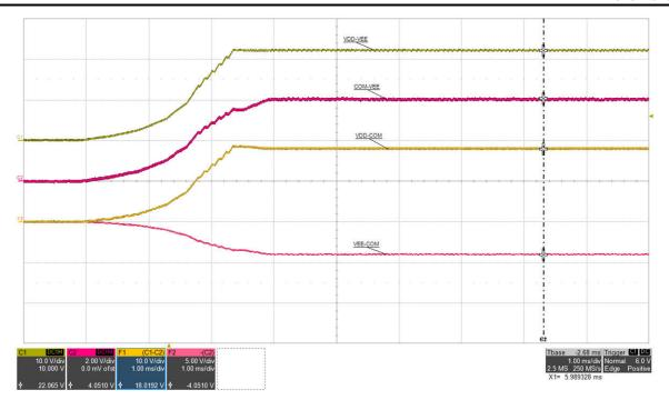
Figure 5-6. Start-up 2: VIN=15 V, I<sub>VDD-VEE</sub>=68 mA, (top: VDD-VEE, 10 V/div, mid-1: COM-VEE, 2 V/div, mid-2: VDD-COM, 10 V/div, bot: VEE-COM, 5 V/div), time = 1 ms/div
