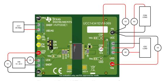
Figure 4-1. Typical Efficiency Measurement Setup
