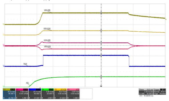
Figure 5-21. Output UVLO: Vin=15 V, PVDD=0 mW, PVEE=50 mW, (top: VDD-VEE, 20 V/div, mid-1: VDD-COM, 50 V/div, mid-2: COM-VEE, 5 V/div, mid-3: VEE-COM, 5 V/div, mid-4: RLIM, 20 V/div, bot: /PG, 5 V/div), time = 5 ms/div
