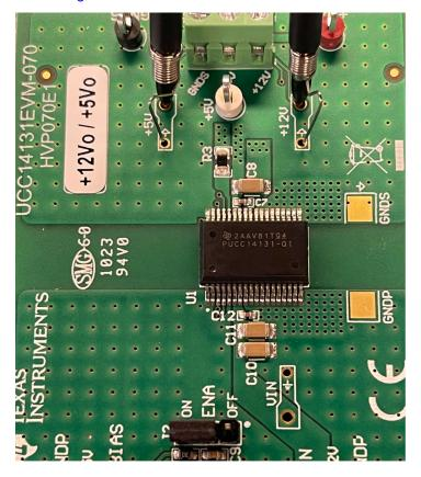
Figure 4-2. UCC14131EVM-070, PCB Scope Probe Test Points
