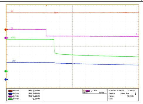
Figure 3-4. LM74912-Q1 Shutdown With EN - HGATE and Output Voltage Profile
