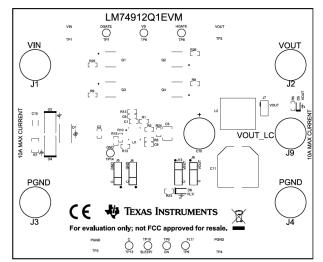
Figure 4-2. LM74912Q1EVM Board Top Overlay
