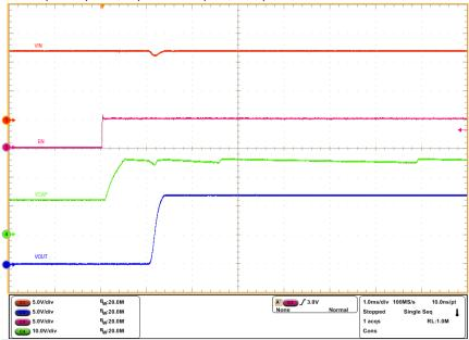
Figure 3-2. LM74912-Q1 Start-Up With EN - Charge Pump and Output Voltage Profile
