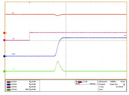
Figure 3-3. LM74912-Q1 Start-Up With EN - Output Voltage and Input Current Profile
