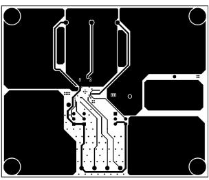
Figure 4-7. LM74912Q1EVM Board Inner Layer 2
