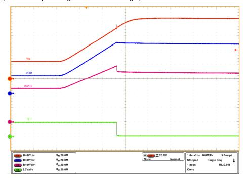
Figure 3-6. Overvoltage Protection
