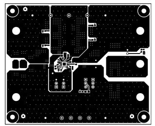
Figure 4-4. LM74912Q1EVM Board Top Layer
