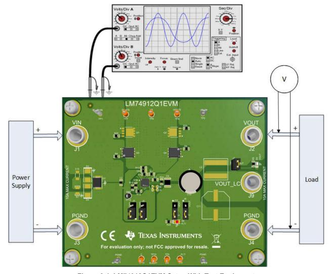
Figure 3-1. LM74912Q1EVM Setup With Test Equipment
