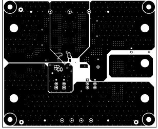
Figure 4-5. LM74912Q1EVM Board Bottom Layer
