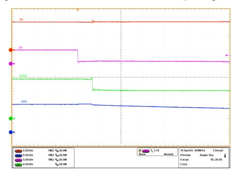
Figure 3-5. LM74912-Q1 Shutdown With EN - DGATE and Output Voltage Profile
