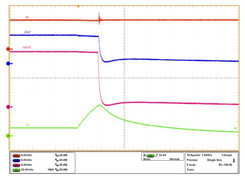
Figure 3-7. Output Hot-Short Response of LM74912-Q1 Device
