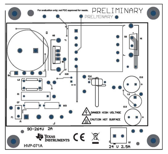
Figure 4-2. EVM Assembly (Top View)
