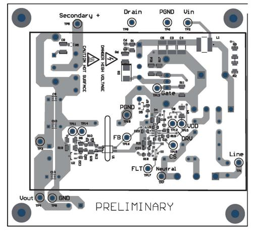
Figure 4-3. EVM Assembly/Layout (Bottom View)
