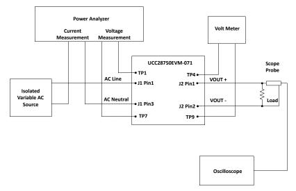
Figure 2-1. UCC28750EVM-001 Test Setup Diagram
