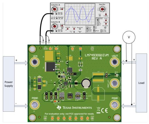
Figure 2-1. LM74930Q1EVM Setup With Test Equipment
