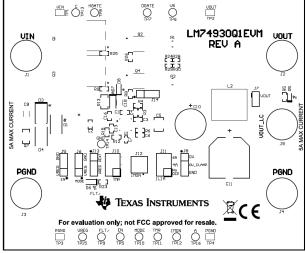
Figure 3-2. LM74930Q1EVM Board Top Overlay
