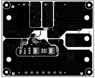
Figure 3-5. LM74930Q1EVM Board Bottom Layer
