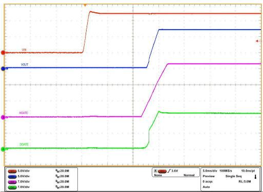
Figure 2-2. LM74930-Q1 Start-Up With VIN - HGATE, DGATE and VOUT
