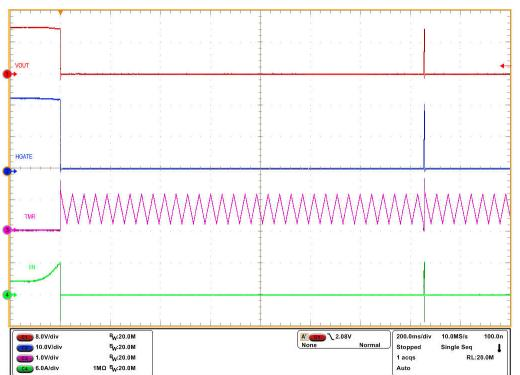
Figure 2-6. Auto-Retry Response of LM74930-Q1 for an Overcurrent Fault
