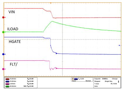
Figure 2-7. Output Hot-Short Response of LM74930-Q1 Device
