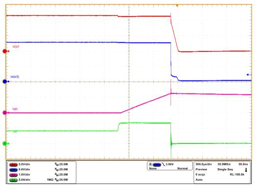
Figure 2-5. Overcurrent Response of LM74930-Q1 for a Load Step From 3.8 A to 6 A With 4-A Overcurrent Protection Setting
