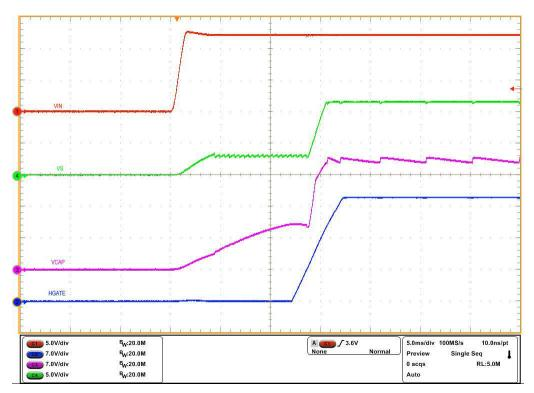
Figure 2-3. LM74930-Q1 Start-Up With VIN - VS, CAP and HGATE
