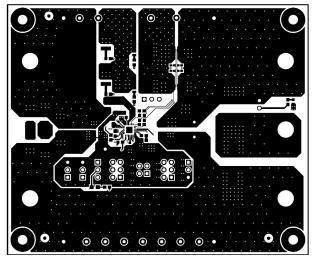
Figure 3-4. LM74930Q1EVM Board Top Layer
