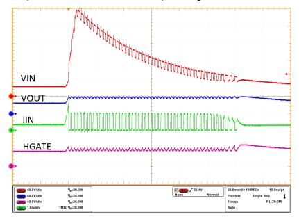
Figure 2-4. Unsuppressed Load Dump 200 V - Output Clamp (OVCLAMP = GND)
