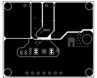
Figure 3-6. LM74930Q1EVM Board Inner Layer 1
