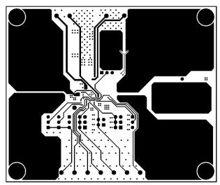
Figure 3-7. LM74930Q1EVM Board Inner Layer 2
