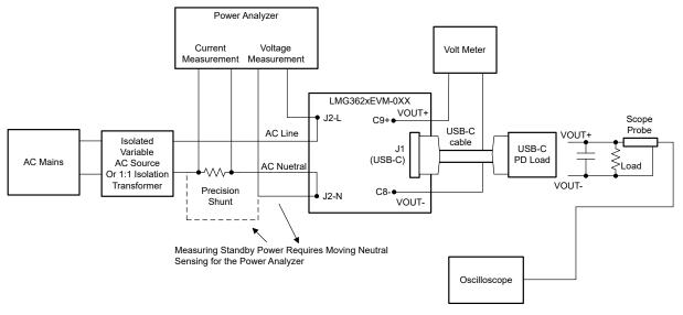
Figure 3-1. LMG3624EVM-081 Test Setup Diagram
