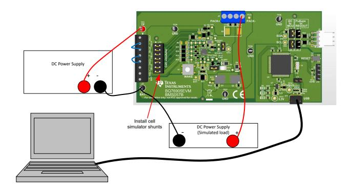
Figure 2-3. Simulating Current Setup
