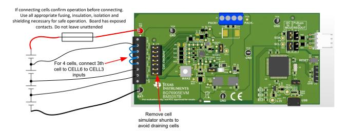
Figure 2-5. Example Connection with 4 Cells
