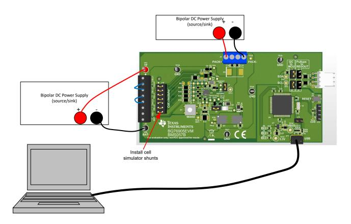
Figure 2-2. Evaluating with Charge or Discharge Current
