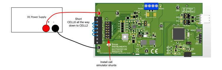
Figure 2-4. Example 3 Cell Simple Evaluation Configuration
