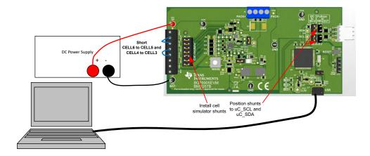
Figure 3-1. EVM Connection for Basic Operation
