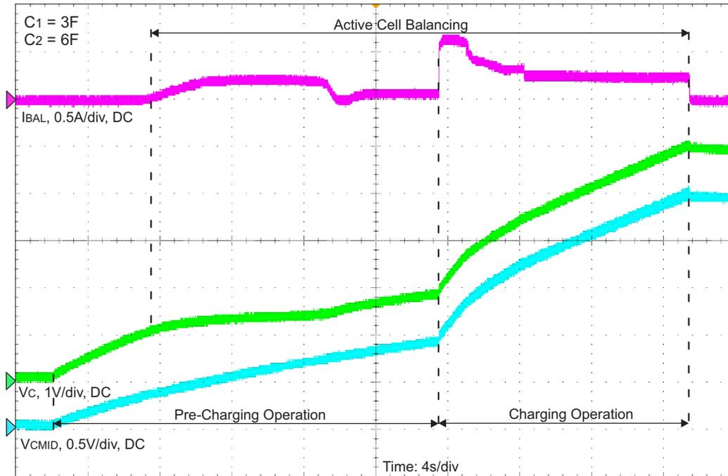
Figure 8. Cell Balancing Operation During Charge Operation
