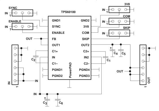
Figure 1–1. Schematic of the Evaluation Module (EVM)
