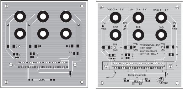
Figure 1–4. Top Layer of the Interface Card, and Placement of Components
