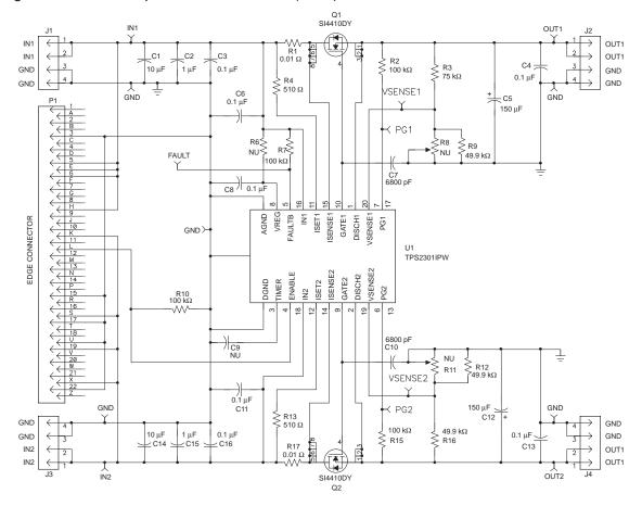
Figure 1–1. Hot-Swap Evaluation Module (EVM) Schematic
