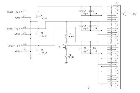
The figures show that the hot-swap EVM board has two supply inputs: IN1 and IN2; but the interface board has three supplies available. VIN3 on the interface board is not used for the evaluation of the dual hot-swap EVM board.
