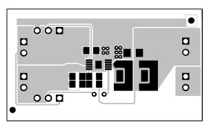
Figure 3-4 shows the PCB layout bottom layer
