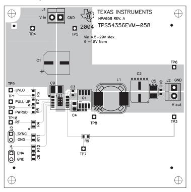
Figure 3–4. Bottom Side Assembly (looking from top side)
