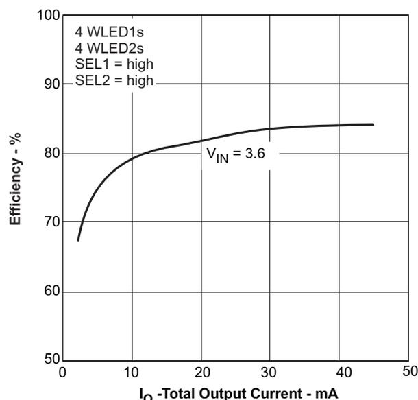
Figure 2. Both On Efficiency vs. Total Output Current
