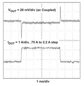
Figure 4. Load Transient Response
