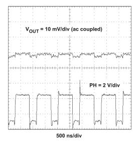
Figure 6. Measured Output Voltage Ripple
