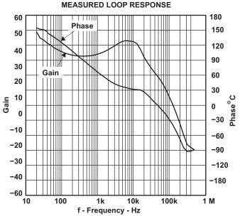
Figure 5. Measured Loop Response
