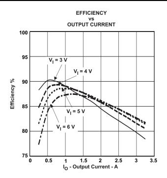
Figure 1. Measured Efficiency
