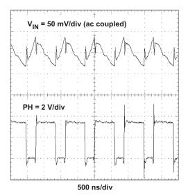
Figure 7. Input Voltage Ripple
