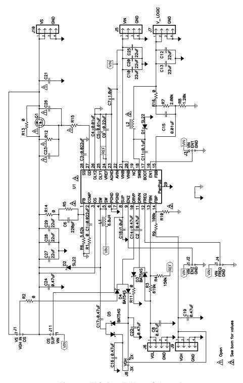
Figure 7. TPS65161EVM-194 Schematic
