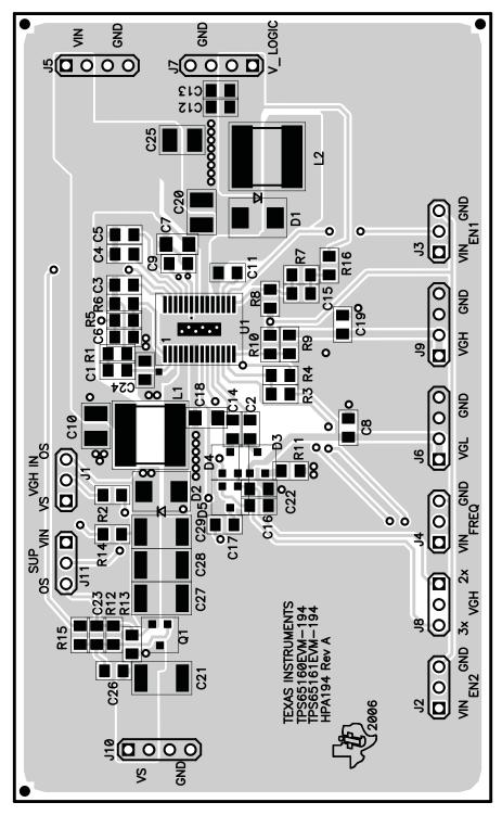
Figure 4. Top Assembly Layer
