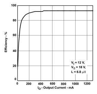
**Figure 1. Boost Converter Efficiency**
