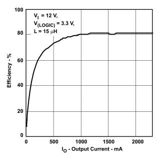
Figure 2. Buck Converter Efficiency
