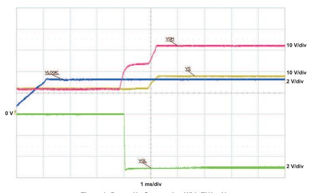
Figure 3. Power-Up Sequencing With EN2 =  $V_{IN}$
