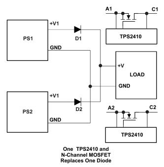
Figure 1. Conventional Wire-OR Power Supplies
