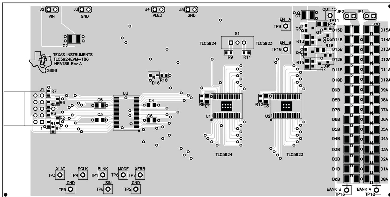
Figure 2. Assembly Layer
