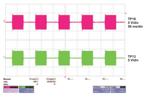
Figure 6. Internal Burst Dimming 50%, BBR Pin at 1 V
