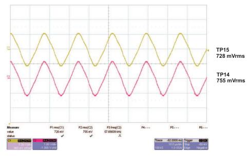
Figure 1. Lamp 1 and Lamp2 VSEN Test Points
