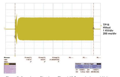
Figure 7. Open-Lamp Shutdown, Time 1.65 Seconds, Lamp 1 Voltage
