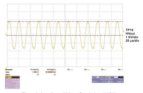
Figure 8. Open-Lamp Voltage Regulation, 1295 Vrms
