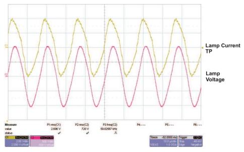
Figure 2. Lamp 1 VSEN Test Point and Lamp 1 Voltage
