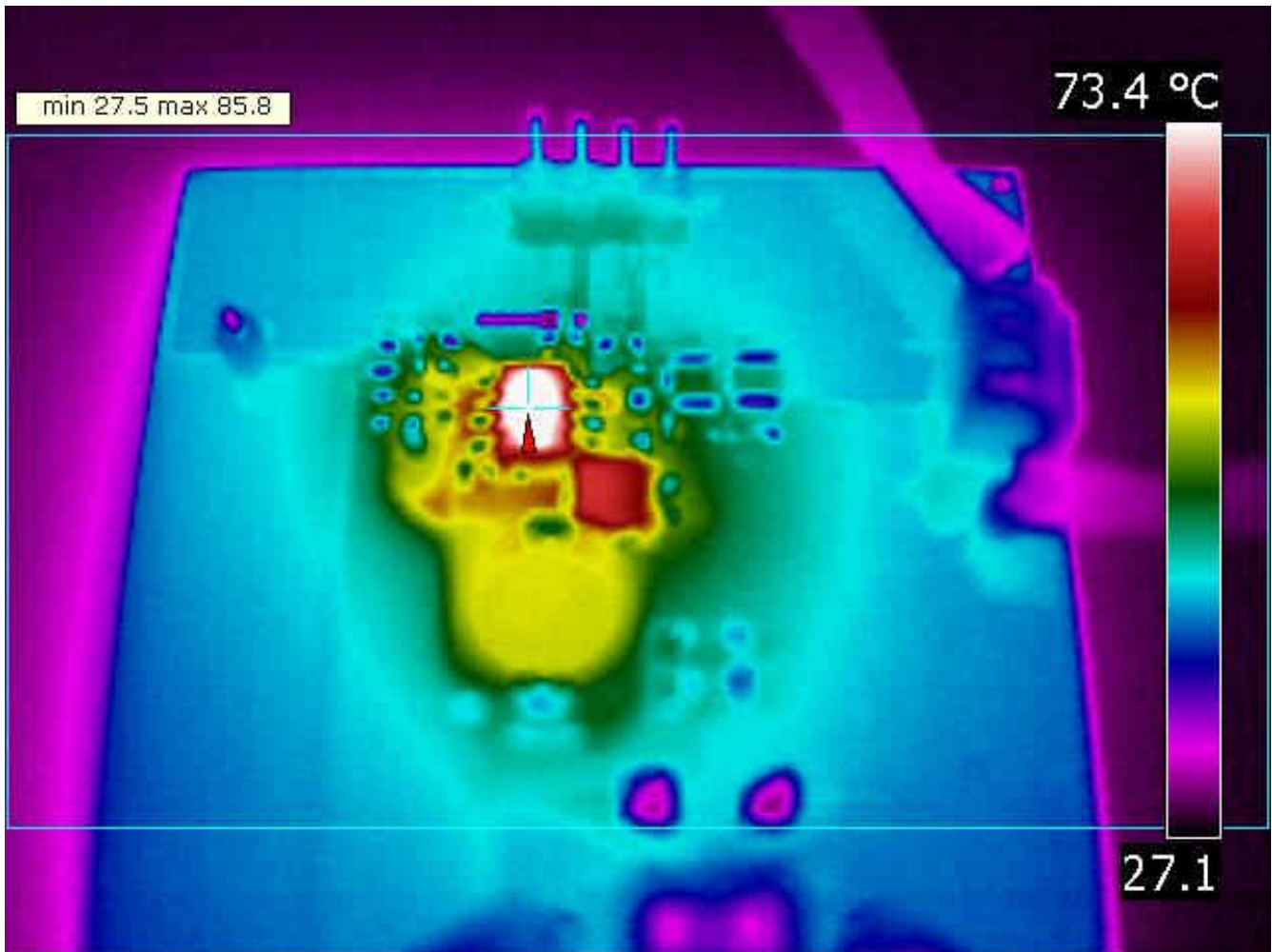
Figure 2-12. TPS54231EVM-372 Thermal Image
