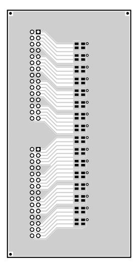
Figure 12. Top Layer Routing
