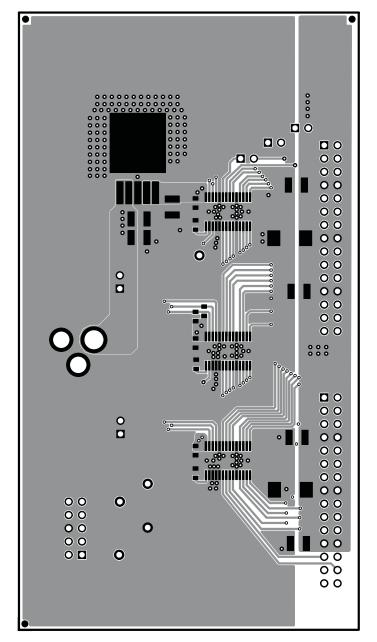
Figure 7. Top Layer Routing
