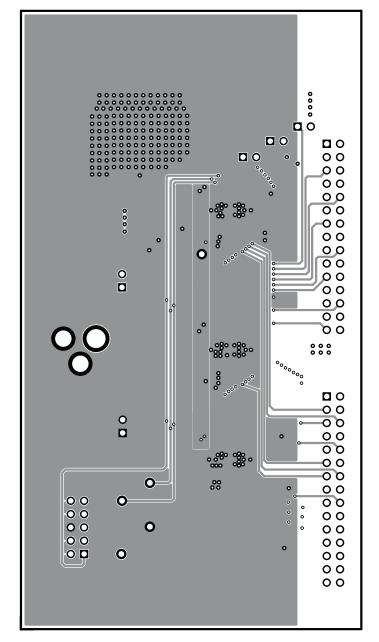
Figure 9. Layer 3 Routing
