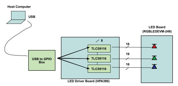
Figure 1. Driver Board and LED Board Connections
