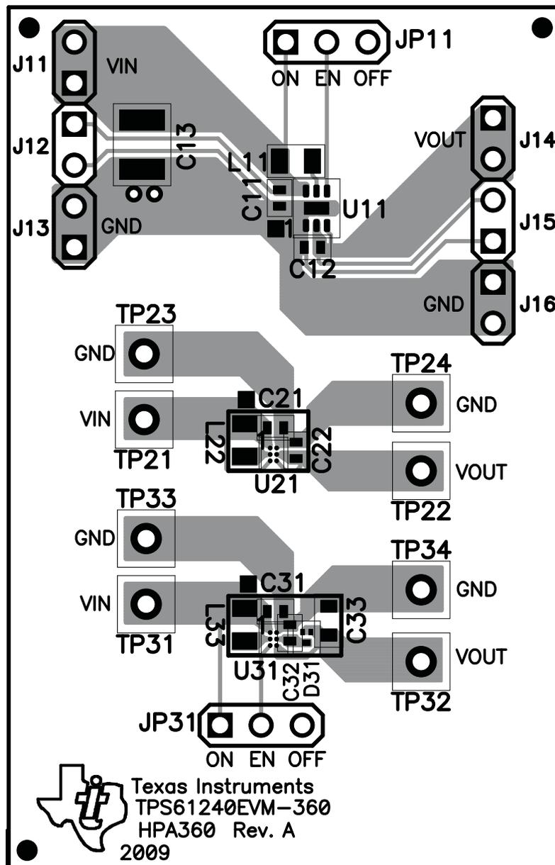
Figure 1. Assembly Layer
