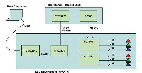
Figure 1. Board Connections
