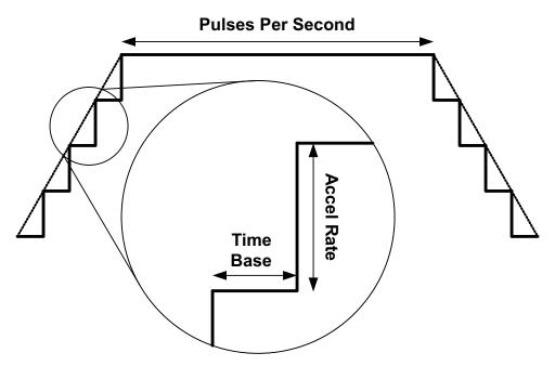
Figure 25. Turning the Stepper Motor
