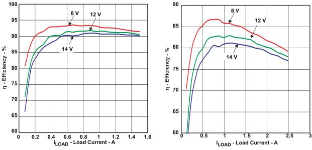
$V_{IN}$  = 9.6-13.2V,  $V_{OUT1}$  = 3.3V  $I_{OUT1}$  = 0-1.5A,  $V_{OUT2}$  = 1.2V  $I_{OUT2}$  = 0-2.5A
