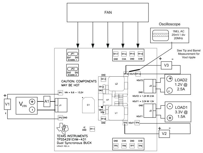
Figure 4-1. TPS54291EVM-431 Recommended Test Setup
