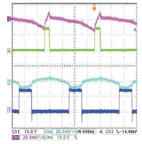
V<sub>IN</sub> = 13.2 V, V<sub>OUT1</sub> = 3.3 A, I<sub>OUT2</sub> = 1.2 V I<sub>OUT2</sub> = 2.5 A Ch1: TP3 (VOUT1), Ch2: TP18 (VOUT2), Ch3: TP9 (SW1), Ch4: TP12 (SW2)
