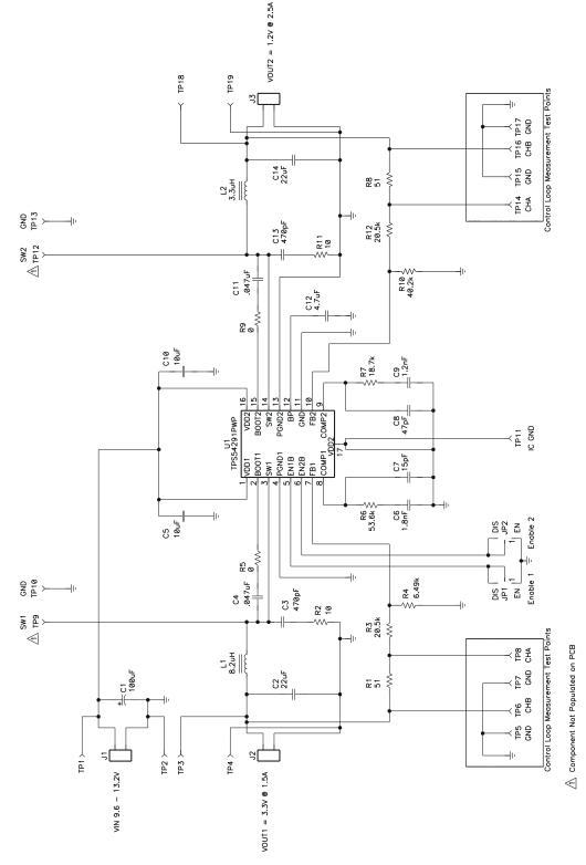
Figure 3-1. TPS54291EVM-431 Schematic
