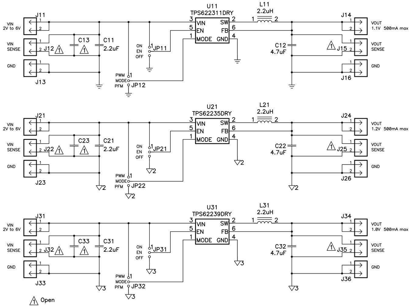
Figure 4. TPS62239EVM-574 Schematic
