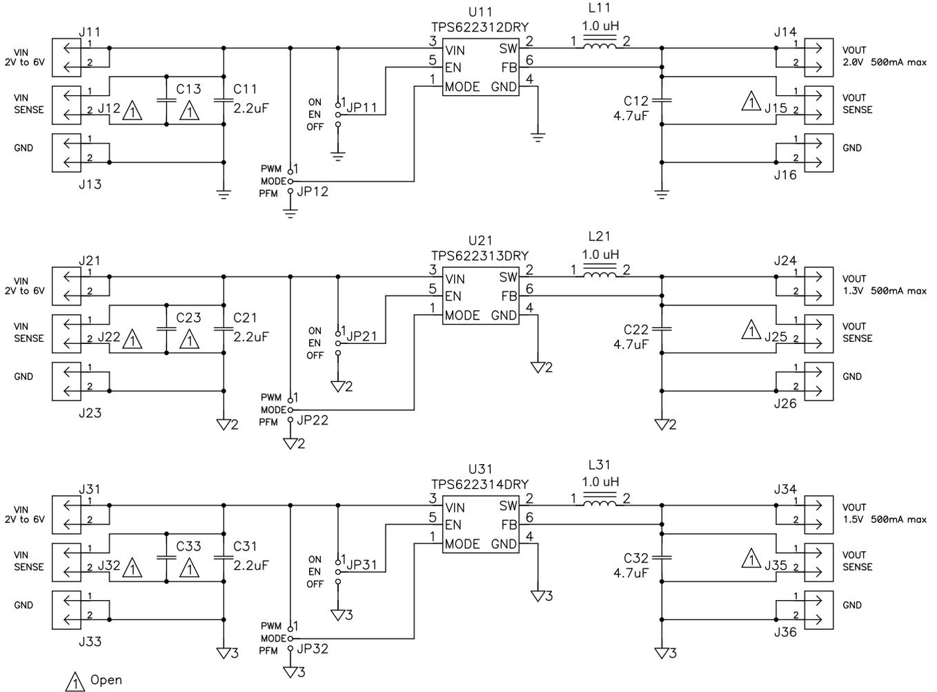
Figure 4. TPS622312/13/14EVM-574 Schematic
