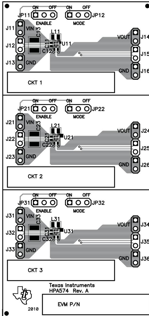
**Figure 1. Assembly Layer**
