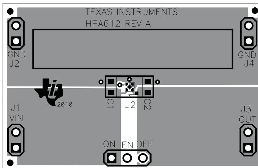
**Figure 3. Assembly Layer**
