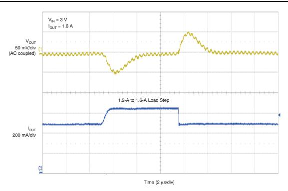
Figure 15. TLV62065 Transient Response, PWM Mode
