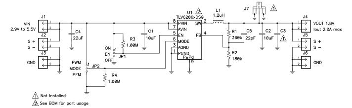
Figure 1. TLV62065EVM Schematic
