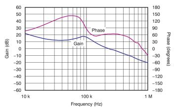
Conditions: VIN = 5 V, VOUT = 1.8 V,  $I_{OUT}$  = 1.6 A; bandwidth: 241 kHz, phase margin: 66°
