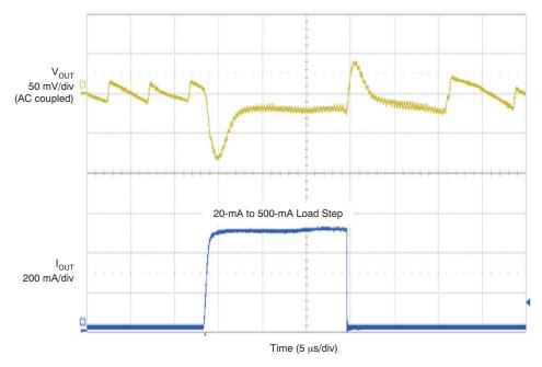
Figure 14. TLV62065 Transient Response, PFM Mode
