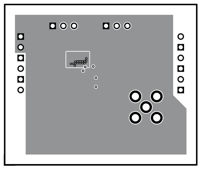
Figure 19. TLV62065EVM Internal Layer 2, X-Ray View From Top
