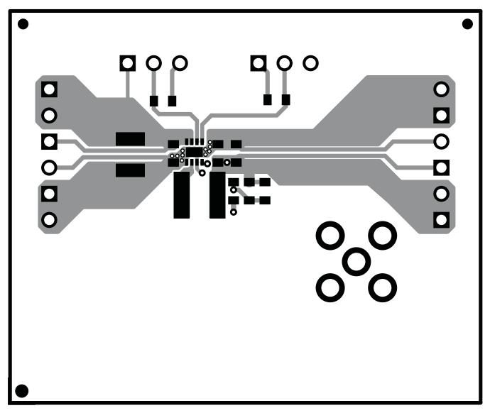
Figure 17. TLV62065EVM Top-Side Copper, Top View
