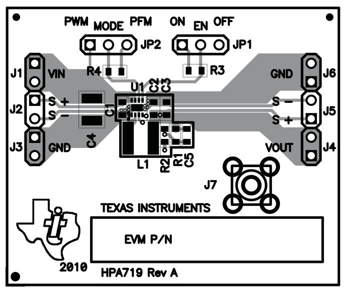
Figure 16. TLV62065EVM Component Placement, Top View
