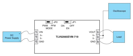
Figure 2. Hardware Board Connection
