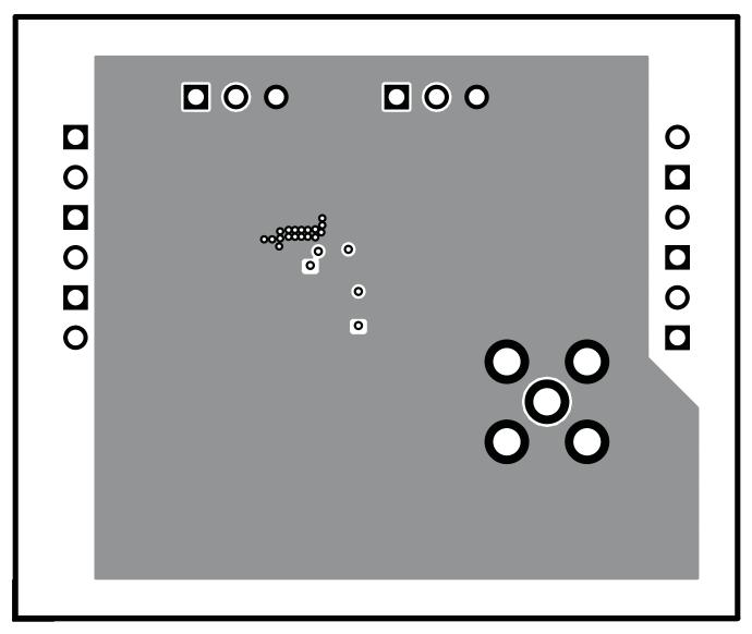
Figure 18. TLV62065EVM Internal Layer 1, X-Ray View From Top
