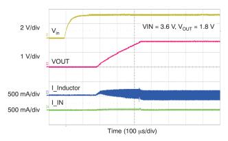
Figure 6. TLV62065 Start-up With No Load
