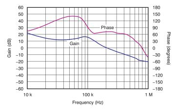
Conditions: VIN = 3.6 V, VOUT = 1.8 V,  $I_{OUT}$  = 1.6 A; bandwidth: 213 kHz, phase margin: 73°
