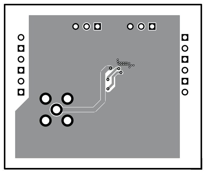
Figure 20. TLV62065EVM Bottom-Side Copper, Bottom View
