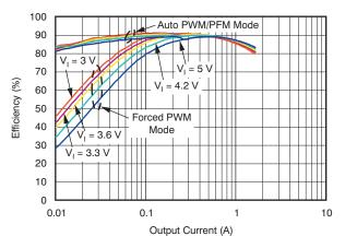
Figure 4. TLV62065 Efficiency vs Load Current
