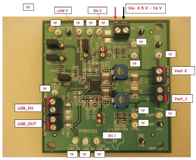
Figure 7. Headers Description and Jumper Placement
