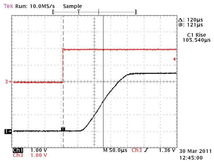
Figure 6. TPS22924B TON and Trise Example
