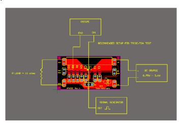
Figure 2. Slew Rate Setup
