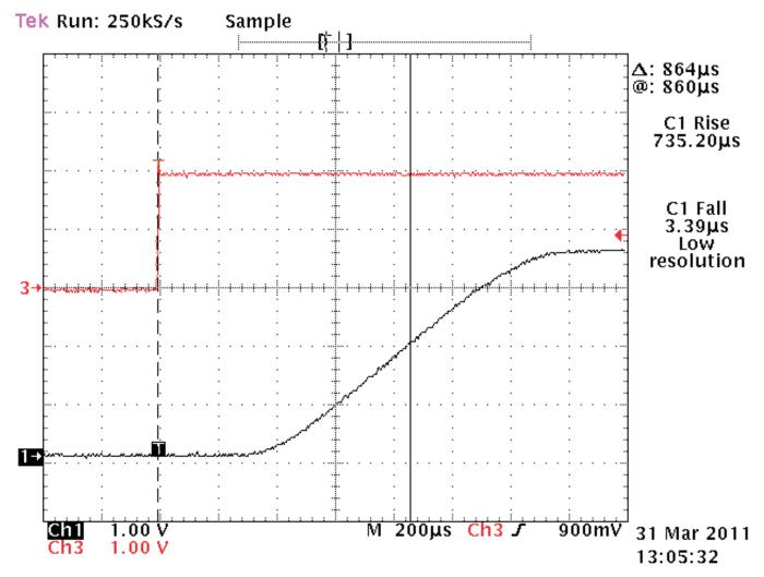
Figure 7. TPS22924C TON and Trise Example
