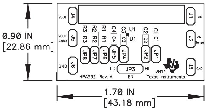
Figure 3. Top Assembly Layer
