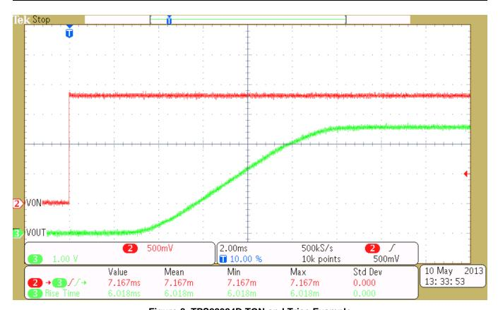
Figure 8. TPS22924D TON and Trise Example
