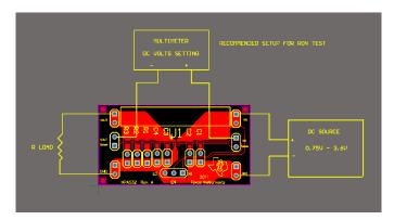
Figure 1. r<sub>on</sub> Setup
