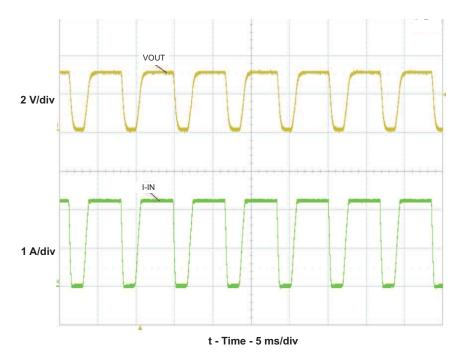
Figure 10. TPS2069CDGNEVM-635 Short-Circuit Input Current and Output Voltage
