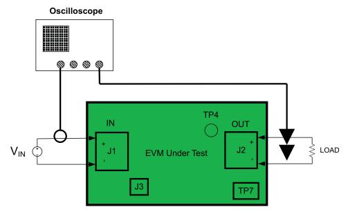
Figure 9. EVM Setup For Measuring Current Limit
