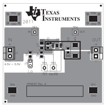
Figure 6. TPS20xxCDGNEVM-635 Component Placement
