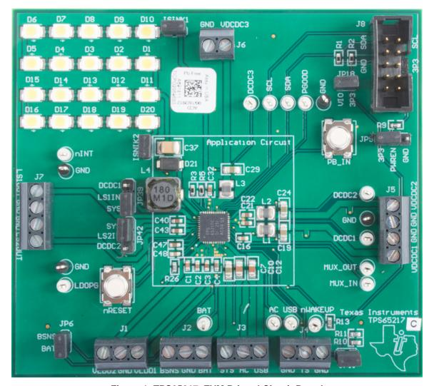
Figure 1. TPS65217xEVM Printed Circuit Board
