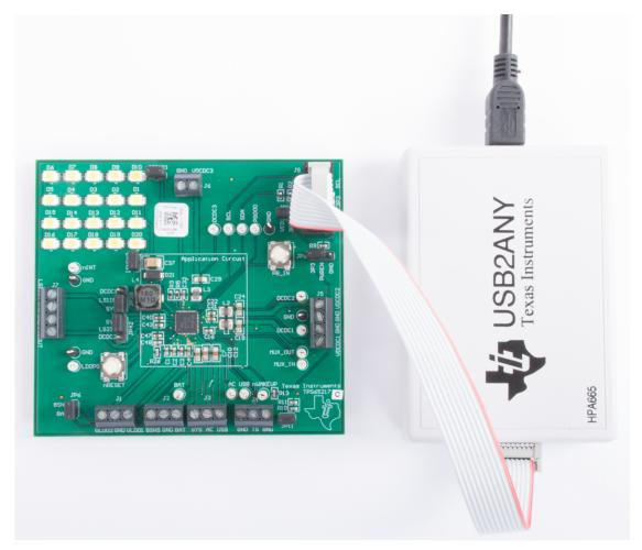
Figure 4. TPS65271 EVM and USB2ANY Connected for Using the IPG-UI Software
