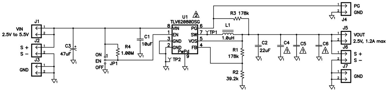
Figure 9. Schematic
