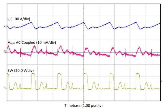
Figure 9. TPS55340EVM-017 DCM Output Ripple
