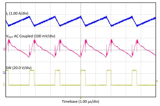
Figure 7. TPS55340EVM-017  $V_{IN}$  = 5-V Output Ripple
