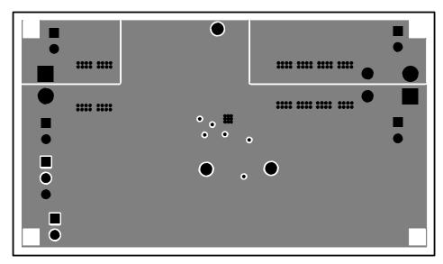
Figure 19. TPS55340EVM-017 Internal Layer-1 Layout
