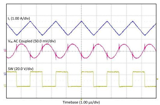
Figure 12. TPS55340EVM-017 V<sub>IN</sub> = 12-V Input Voltage Ripple
