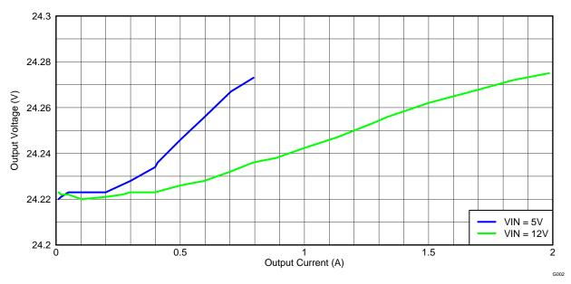
Figure 2. TPS55340EVM-017 Output Voltage Load Regulation
