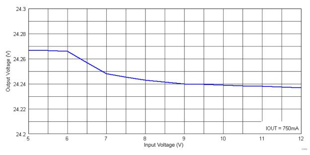
Figure 3. TPS55340EVM-017 Output Voltage Line Regulation
