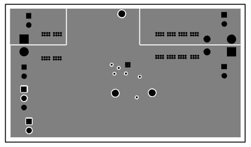
Figure 20. TPS55340EVM-017 Internal Layer-2 Layout
