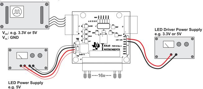
Figure 2. TLC59282 EVM Recommended Test Set-Up
