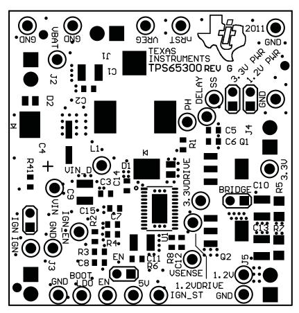
Figure 7. Top Assembly Layer
