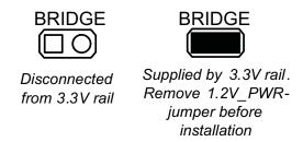
Figure 6. Bridge Jumper Settings
