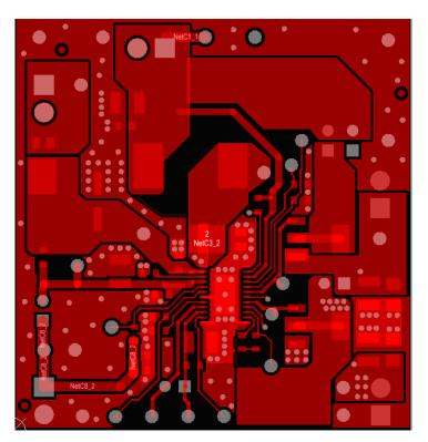
Figure 8. Top Layer Routing
