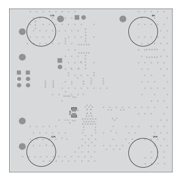
Figure 3. Component Placement, Bottom Overview
