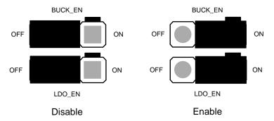
Figure 7. Enable Jumper Setting
