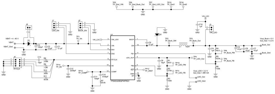
Figure 1. TPS65320EVM Schematic
