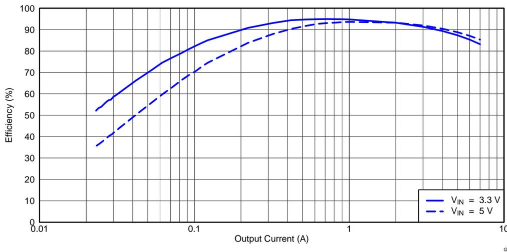
**Figure 2. TPS54719EVM-152 Low Current Efficiency**
