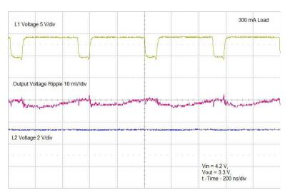
Figure 4. Output Ripple Vin 4.2 V
