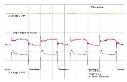
Figure 3. Output Ripple Vin 2.2 V
