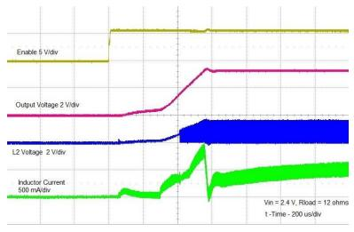
Figure 1. Turn ON into Load, Vin = 2.4 V
