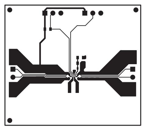
Figure 7. Top Layer Routing
