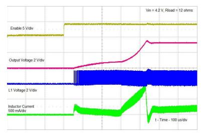
Figure 2. Turn ON into Load, Vin = 4.2 V
