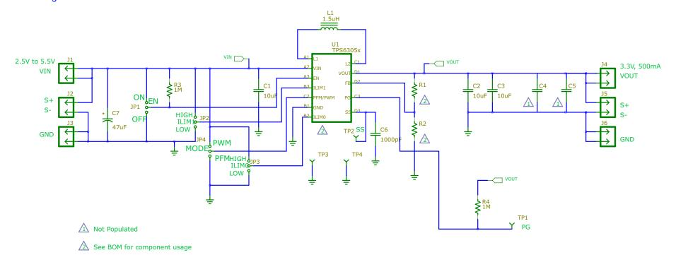
Figure 5. TPS6305xEVM-180 Schematic
