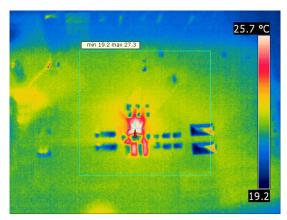
Figure 1. Thermal Performance (Vin = 5.5 V, Load = 500 mA)
