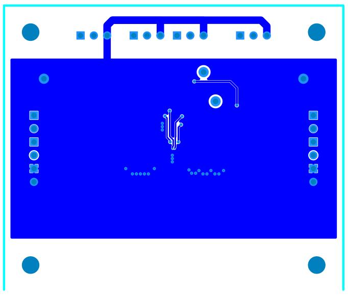
Figure 4. Bottom Layer Routing
