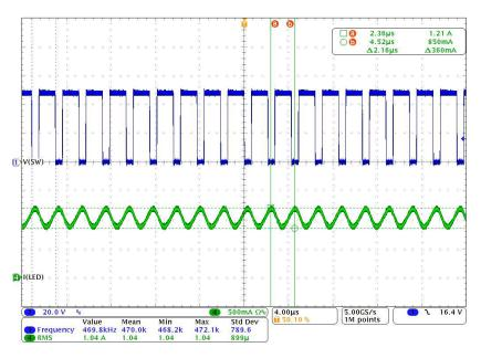
10 serial LEDs,  $T_A = 25^{\circ}C$ I<sub>LED</sub>: 500 mA/DIV, V<sub>SW</sub>: 20 V/DIV
