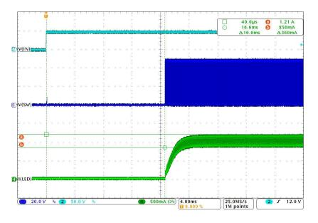
10 serial LEDs,  $T_{A}{=}25^{\circ}\text{C}$  I\_{LED}: 500 mA/DIV, V\_{SW}{:} 20 V/DIV, V\_{IN}{:} 50 V/DIV
