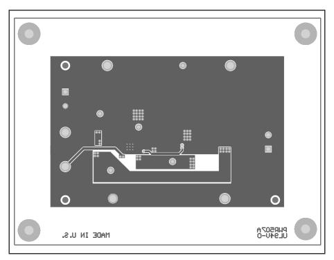
Figure 9. TPS92641EVM PCB Bottom View
