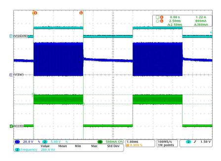
10 serial LEDs,  $T_A = 25^{\circ}C$ I<sub>LED</sub>: 500 mA/DIV, V<sub>UDIM</sub>: 5 V/DIV, V<sub>SW</sub>: 20 V/DIV
