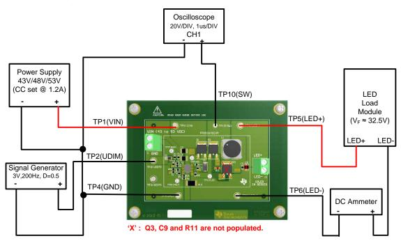
Figure 3. Test Connection Diagram of the TPS92641EVM
