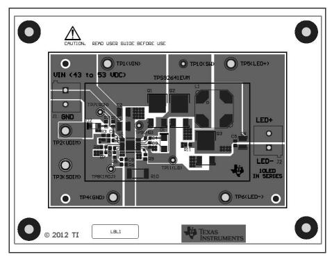
Figure 7. TPS92641EVM PCB Top View with Component Legend
